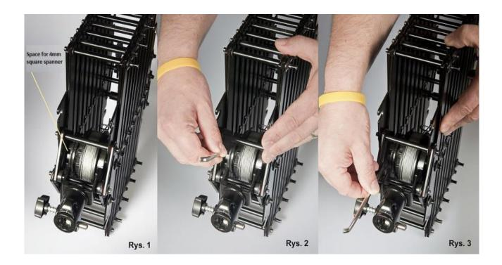
Tension is to be set experimentally on the principle of "small steps" by doing a small turnover and checking whether the pantograph works properly.
