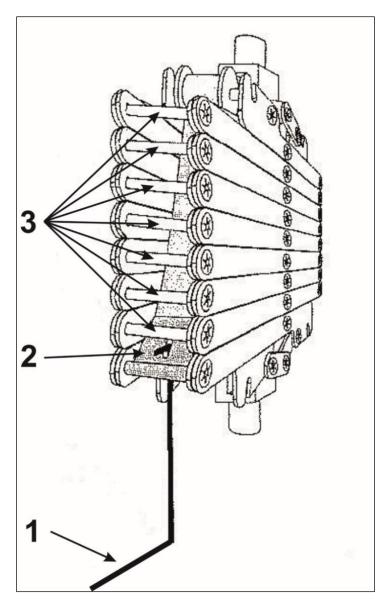
that is to be mounted on the pantograph. The spring tension is adjusted by hooking the spring holder (element 2) to the corresponding bar (element 3). The more distant bar is chosen for the holder to be hooked the more weight is balanced.
