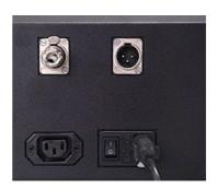
Pic. 4 Power supply sockets with main switch and DMX 512 plugs
